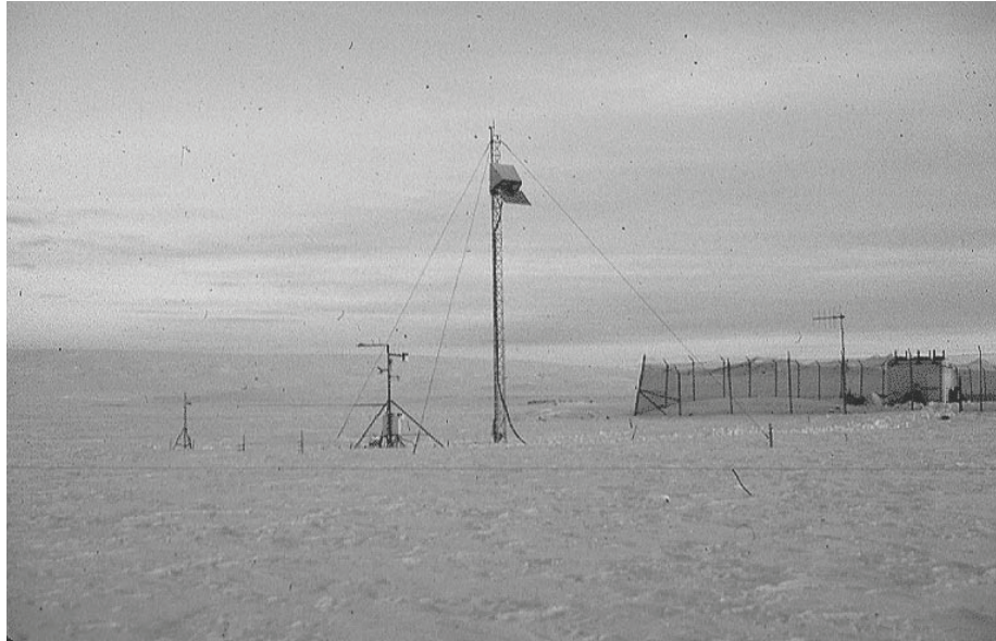
Figure 1. REBEX-3 tundra site photo in January. Microwave radiometers are at the top of the tall 10-meter tower. Meteorological instruments are to the left of the 10-m tower.
