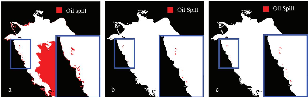
**Figure 1:** Comparison between fix threshold technique (a), RST technique (b) and RST recent development technique (c) in AVHRR channel 4 computed on the Persian Gulf image of 24 January 1991 at 10.31 GMT (13.31 LT). Anomalous pixels are depicted in red, land is masked in black.
