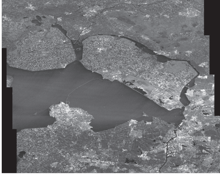
Fig. 2. TOPS acquisition over Flevoland. Azimuth is horizontal and range is vertical, with near range on the top.
