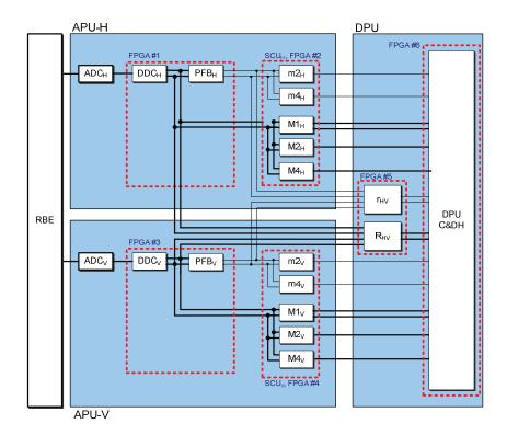
Figure 1: Functional block diagram of SMAP-RDE signal processing chain. The processing is divided into logical modules called the digital downconverter (DDC), Polyphase Filter Bank (PFB) Statistics Calculation unit, and two cross cross correlators. The partitioning of the modules is shown across electronics boards and across FPGA devices.
