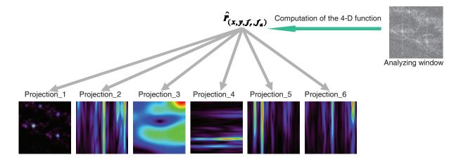
In each projection we obtain an animation showing the variation of target behavior for analysis along with contextual information in different range and azimuth sub-apertures.
