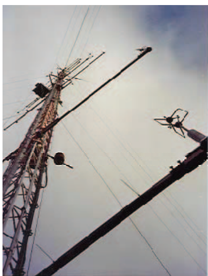
Figure 1. Micro-meteorological tower experiment at Sodankylä (left) and Pallas (right). The 48-m mast at Sodankylä is installed into a Scots pine forests on sandy soil measuring eddy-covariance fluxes of CO 2 , latent and sensible heat and momentum, radiation components, and gradients of the CO 2 concentration, temperature and wind. Soil, vegetation and snow parameters are also monitored in the forest region around the tower. Analogous measurements are carried out for the spruce forest site.
