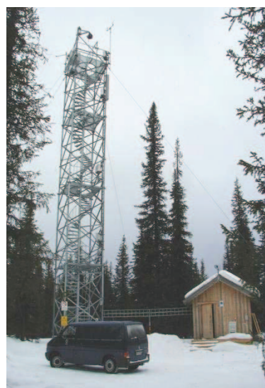
Figure 1. Micro-meteorological tower experiment at Sodankylä (left) and Pallas (right). The 48-m mast at Sodankylä is installed into a Scots pine forests on sandy soil measuring eddy-covariance fluxes of CO 2 , latent and sensible heat and momentum, radiation components, and gradients of the CO 2 concentration, temperature and wind. Soil, vegetation and snow parameters are also monitored in the forest region around the tower. Analogous measurements are carried out for the spruce forest site.
