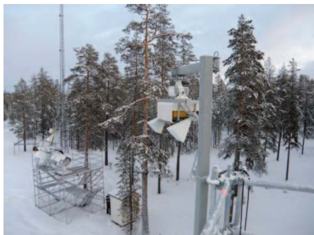
Figure 2. Snow and soil remote sensing reference site at Sodankylä. Left: Instrumentation including the X-Ku-band SnowScat scatterometer (foreground), L-band Elbara-II radiometer and X-, K-, Ka- and W-band SodRad radiometer (back). Right: Overview.
