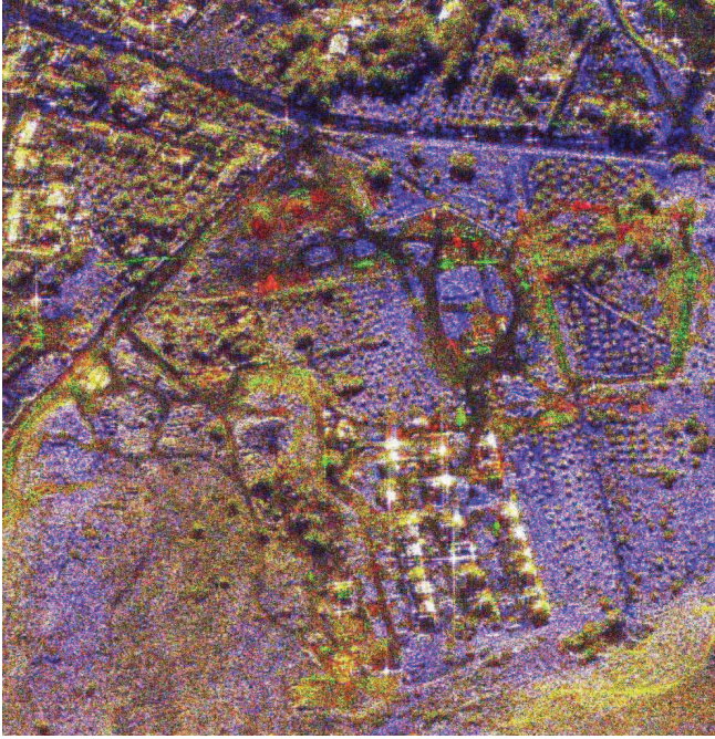
Figure 4 : color composite of sub-metric resolution SAR image: red is the SAR magnitude image of the first acquisition, green is the SAR magnitude image of the second acquisition and blue the coherence magnitude.
