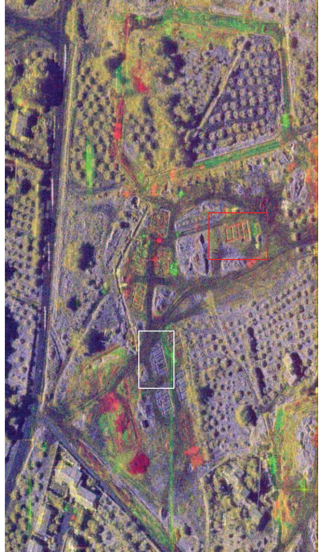
Figure 7: color composite of decimetric resolution SAR image: red is the SAR magnitude image of the first acquisition, green is the SAR magnitude image of the second acquisition and blue the coherence magnitude
