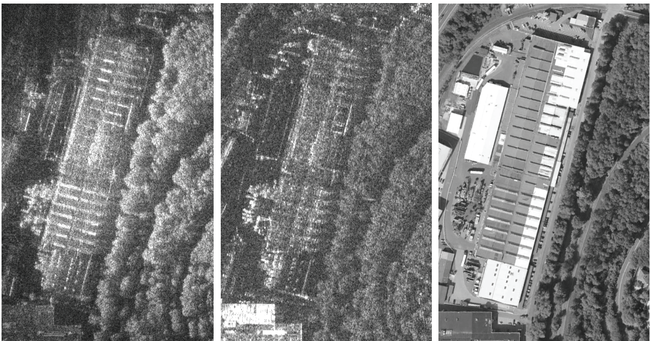
Figure 1: a) Bistatic radar image of a factory obtained with our receiver system b) Monostatic image from TerraSAR-X c) Optical image of the same scene (google earth)
