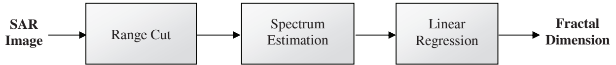
Fig. 2: Block diagram of the extraction of the fractal dimension
