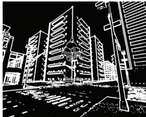
Figure 5: Template building match (note the superimposed damage information)..
