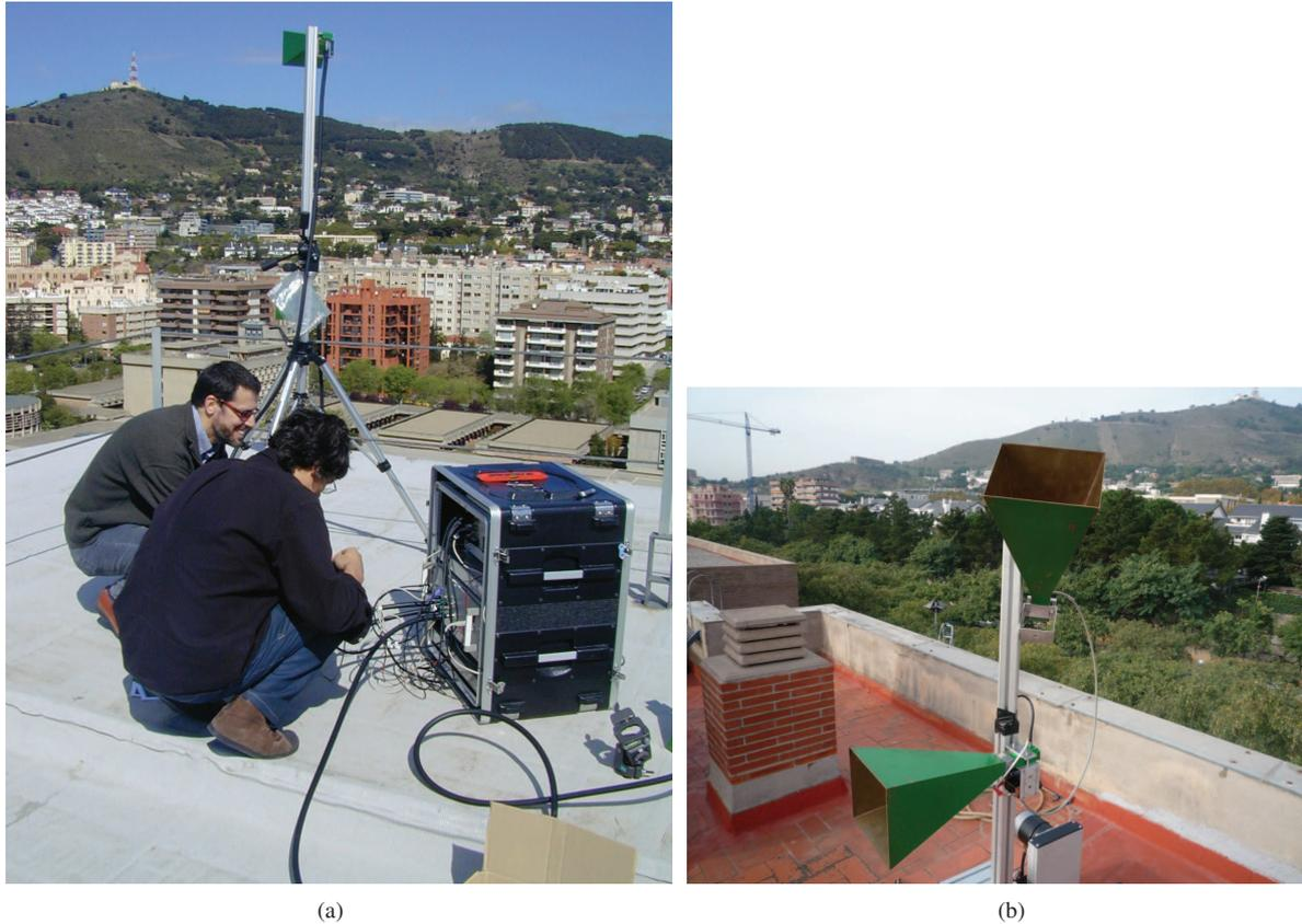
**Fig. 1.** (a) Interferometric set-up with two interferometric channels. (b) Bistatic Active Radar Calibrator (BARC).
