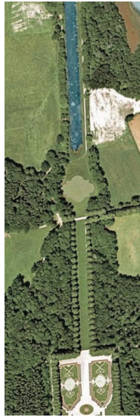
Fig. 1a. FMCW SAR image The processed image has a size of 331 m (Slant range) \times 897 m (Azimuth) at Herrenchiemsee, Germany. (The horizontal and vertical directions denote the range and azimuth, respectively.)
