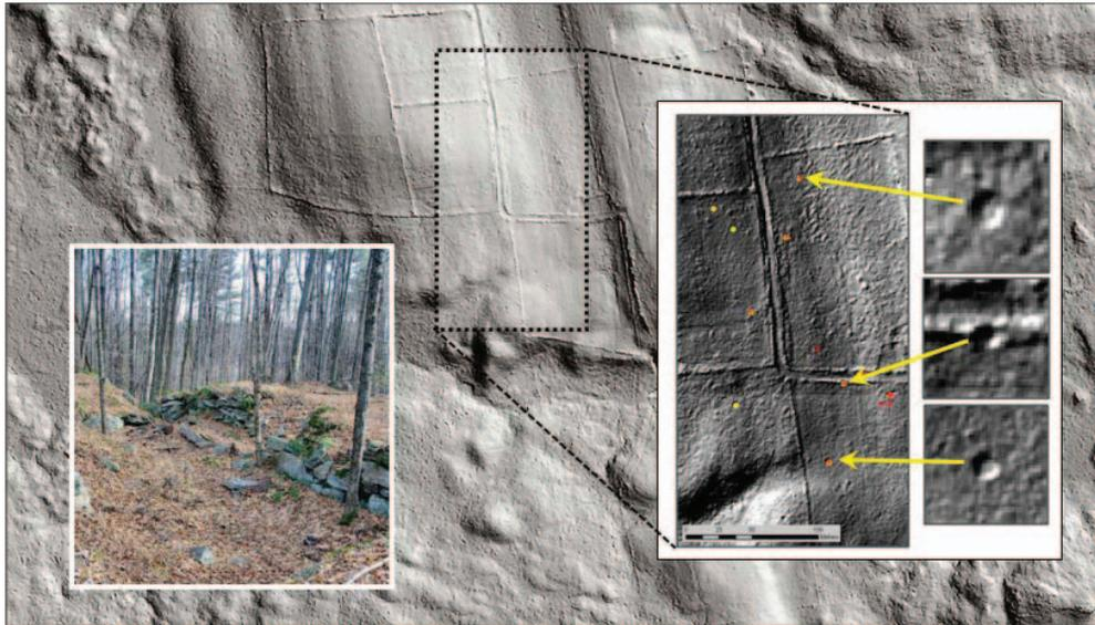
Figure 1. LiDAR is used to produce vegetation and bare earth terrain models to identify munitions related features. Inset-right shows verified craters from prior military training activity.
