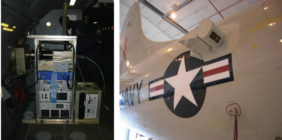
Figure 1. The P3DWL instrument rack is shown on the left and the biaxial scanner is shown on the right along with a fairing form reducing turbulence and drag.
