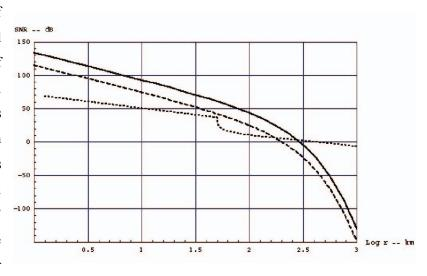
this example the AIS receiving station has an antenna height of 75 m and an AIS antenna height of 15 m aboard a ship. SNR in dB is plotted vs. log of range in km ( $\log r - \text{km}$ ) for HF radar and AIS ship monitoring. The HF radar results are shown for a large ship (10,000 tons) with a solid line and a small ship (120 tons) with a dashed line. AIS receiver results are shown by the dotted line. The intermittent VHF duct is assumed present in this
