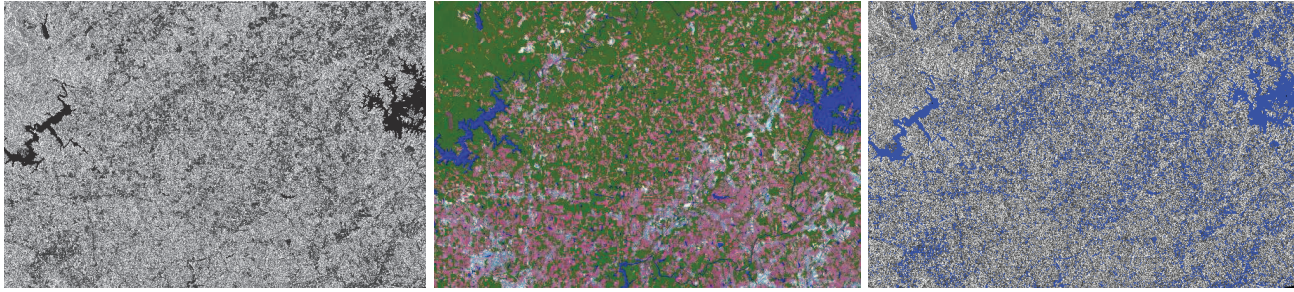
Figure 4. ALOS PALSAR image (left), Landsat image (right), and merged flood distribution (right) for the Georgia floods of September 2009 (ALOS image courtesy the International Charter and JAXA).
