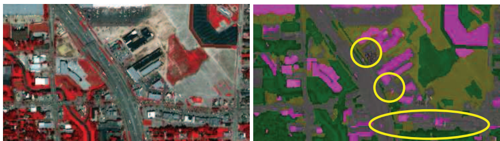
Figure 3. QuickBird image (upper, Houston) and its class map. Misclassification is circled. Image courtesy the International Charter and DigitalGlobe.
