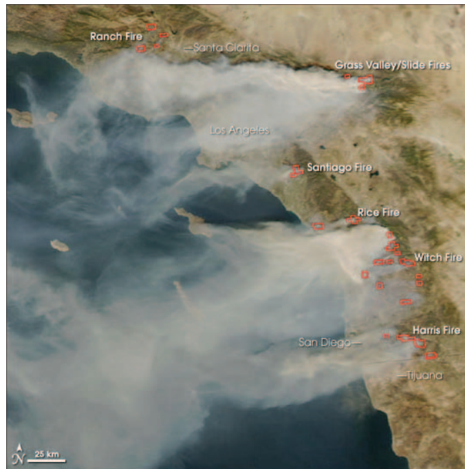
Fig. 1: True color composite of MODIS visible image acquired aboard the Aqua satellite, at 2:40 p.m. Pacific Daylight Time on 23 October 2007 during the Southern California firestorm. The fire locations are delineated with red contours. The grayish thick smoke plumes from the fires are quite prominent. (Image courtesy of the NASA Earth Observatory team: http://earthobservatory.nasa.gov/ ).
