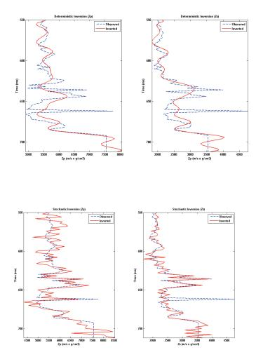
Figure 2: Pre-stack inversion results: Acoustic Impedance (left) and Shear Impedance (right) estimates from a deterministic (top) and fractal based stochastic (bottom) inversion. Note that the stochastic inversion is able to estimate high frequency variations. The red line shows the true well log and the blue is the estimated model.
