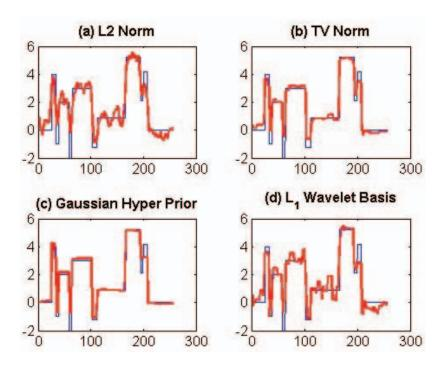
Figure 1: Inversion of seismic data for Acoustic impedance using different regularization techniques. The true model is shown in black while the inverted models are shown in red. Note the superior performance of Gaussian hyperprior compared to other well known regularization methods (modified from Routh et al 2008).
