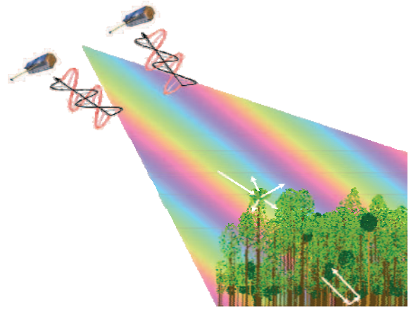
Figure 2: The 3-D structure mode employs polarimetric SAR interferometry to measure tree heights and vertical vegetation profiles. The individual contributions from ground and canopy are separated via their polarimetric signatures and the corresponding heights are measured by cross-track interferometry.
