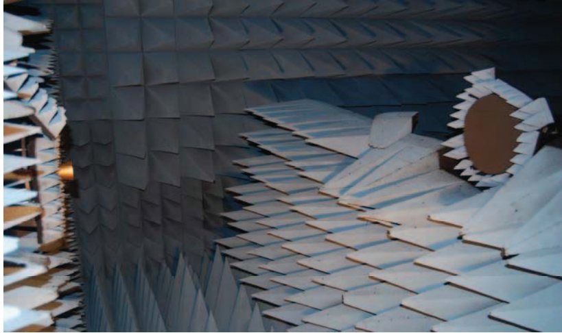
Fig. 1 Measurement setup in anechoic chamber.
