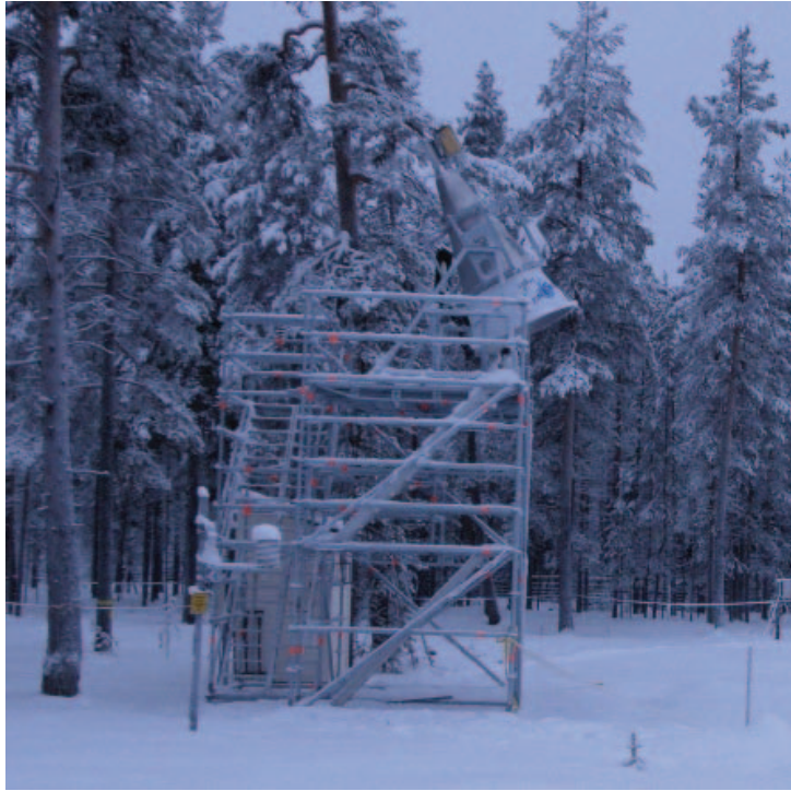
Figure 1: Elbara-II mounted on a 5-m tower (in home position between measurements).
