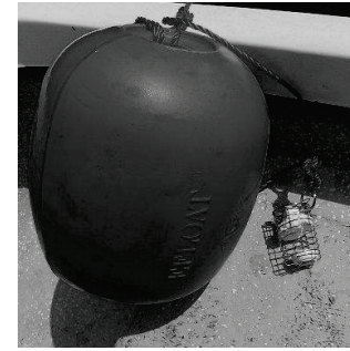
Fig. 3. Photo of a water temperature logger with a float.
