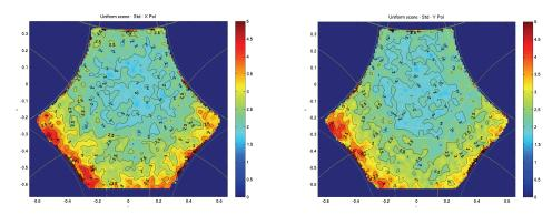
The plots above illustrate the performance assessment of SMOS at brightness temperature map level. These measurements were acquired over south tropical pacific ocean, considered here as uniform and show the temporal standard deviation of the measured brightness temperature within the SMOS field of view. The observed results fall perfectly within the theoretical expected accuracy of around 2.5K at boresight.
