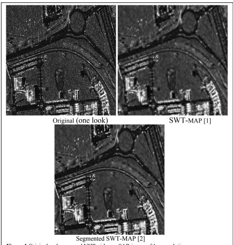
**Figure 1** Original and processed VHR airborne SAR image of 1 m resolution.
