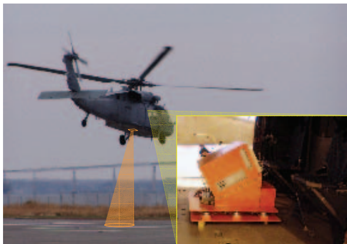
Figure 1: DAMR Instrument Installed in vehicle for initial flight tests.
