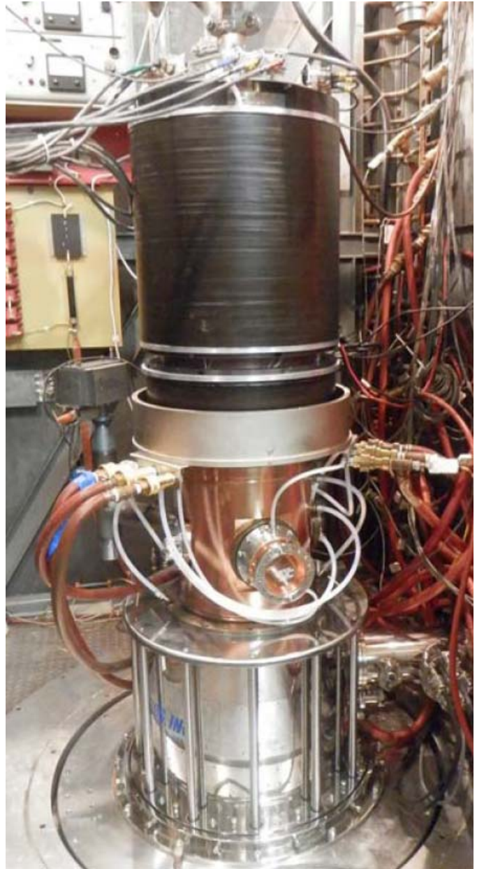
Fig. 1. The VGT-8141 SN2 Gyrotron is installed in the superconducting magnet in CPI's test stand. The system is pictured prior to installation of the output waveguide and load.
