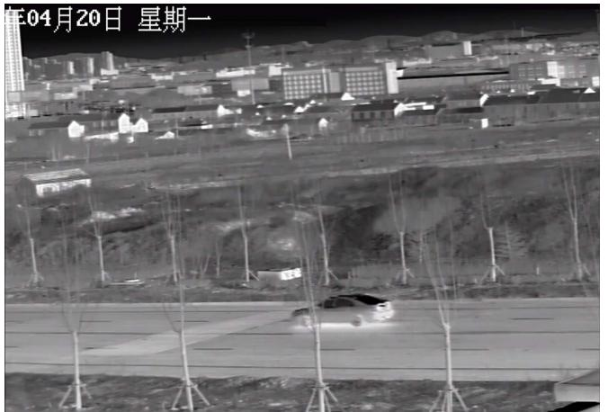
Fig. 7. Thermal image taking with  $17\mu\text{m}$   $640\times 512$  uncooled IRFPAs.
