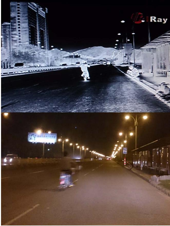
Fig. 8. Thermal image taking with 20 $\mu\text{m}$  384×288 IRFPAs compared to visible image.
