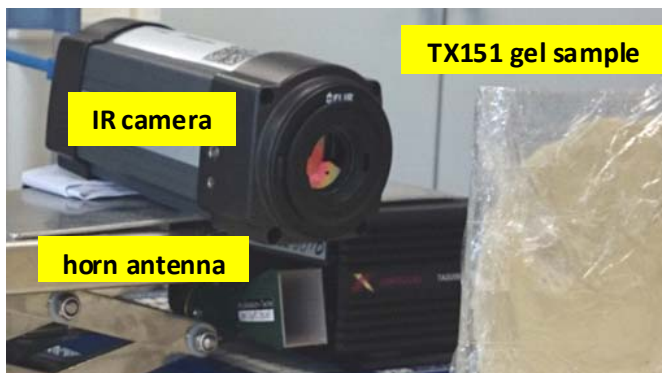
Fig. 1. Exposure setup including horn antenna, IR camera and human skin phantom. The RF generator is not shown here.
