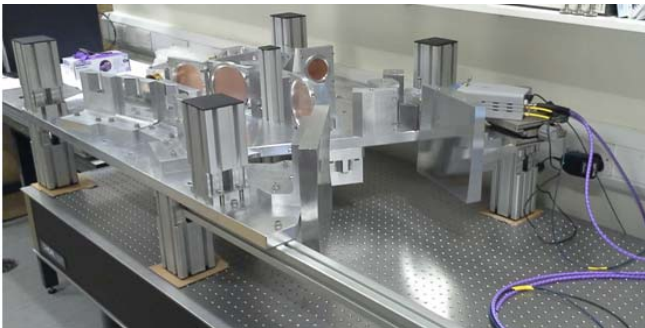
Fig. 1. The doubled layered QOM, with Cu-colored DCPs on the top layer with the VNA head in the top right of the picture.
