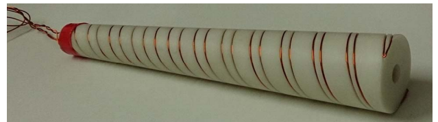
Fig. 1. Photograph of the adiabatically tapered entrance for “improved” short-period wiggler.
