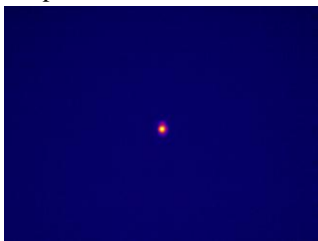
Fig.4. Beam pattern of one pulse from the THz-FEL (3.3 pps)
