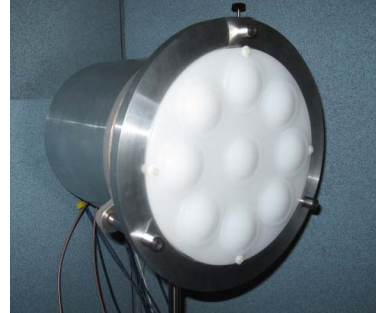
Fig. 1. Front view of sub-THz wave radiating array.
