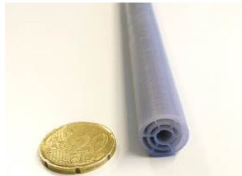
Figure 2. Photograph of a W-band prototype fabricated using 3-D printing.
