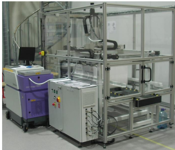
Fig. 1. Terahertz solar crucible inspection system
