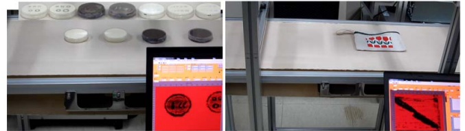
Fig.2. Captured images from the videos demonstrating the capability of the active real-time T-ray imaging system for food inspection (left) and security screening (right). Gaussian beam from the T-ray gyrotron is transformed into a line shape crossing the conveyor belt, where a line array detector placed beneath take the shadow images of the samples moving along the conveyor belt.
