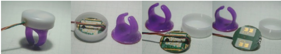
Fig.3: Our finger mount Doppler unit and its exploded views.
