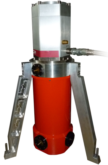
Fig. 1. A detector system (the compressor is not shown; this can be located at a distance as much as 15 m from the cryostat)
