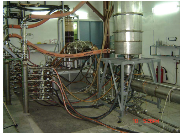
Figure 3. Part of gyrotron setup with water manifold and dummy load.
