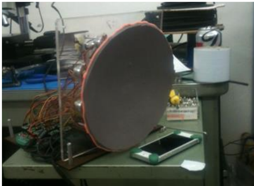
Figure 4. Adaptive corrector prototype. The LBR spherical reflector requires a spherical corrector to bring converging rays to a single focus. The spherical corrector must be adaptive to compensate for nonspherical distortions in the balloon reflector surface. Pictured is an 8 inch scale model prototype of a computer controlled, flexible corrector.
