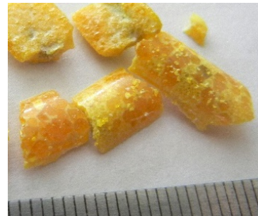
Fig.2. Photograph of polycrystalline Ga 2 S 3 grown by flux method.
