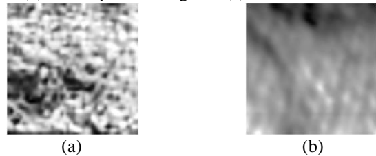
Fig. 1: Effect of rough surface scattering on an image. (a) 0.7 mm spot size and 30 deg. incidence angle. (b) 2.2 mm spot size and 45 deg. incidence angle.
