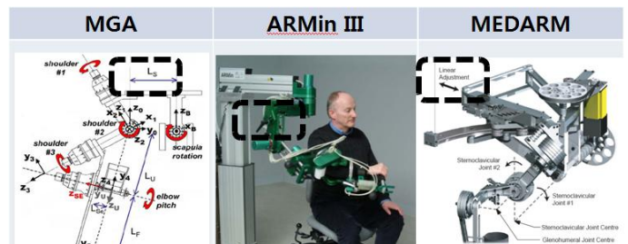
Figure 15. Adjustment part of existing robots
