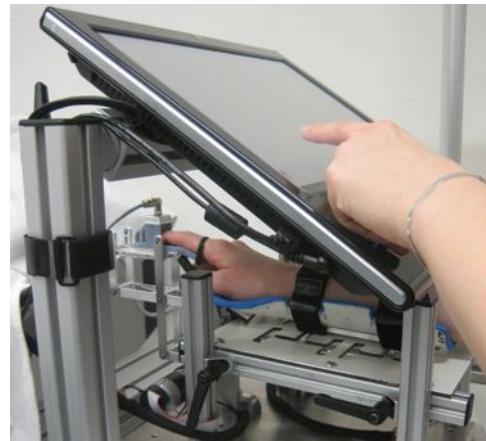
Fig. 1. The Robotic Sensory Trainer for assessment and therapy of hand sensory function. A touch screen computer placed over the interface collects responses from the user and can generate visual and auditory stimuli.
