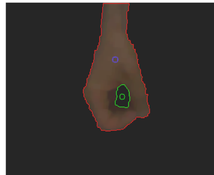
Figure 2: Example of a processed frame (cylindrical grasp, top view), showing the results of the background subtraction, centering, and detection of outer and inner contours.
