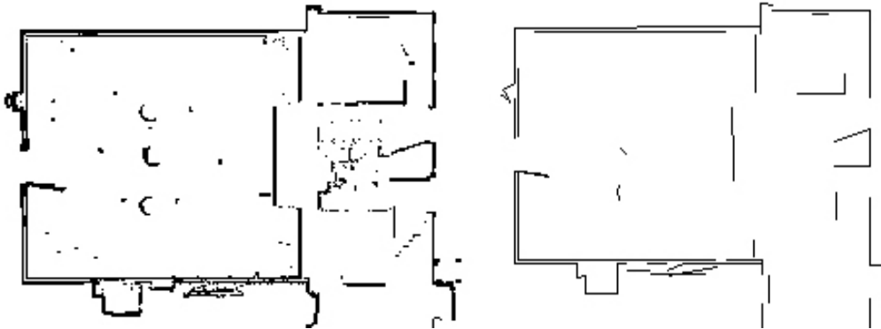
Figure 21. Maps consist of occupancy-grid points (left) and extracted lines (right).
