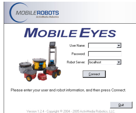
Figure 4. In MobileEyes' startup dialog, enter guiServer's hostname or IP address, not MobileSim's.
