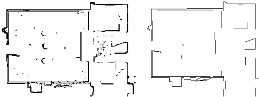
Figure 6. Maps consist of occupancy-grid points (left) and extracted lines (right).
