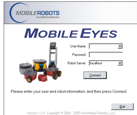
Figure 3. In MobileEyes' startup dialog, enter guiServerSonar 's hostname or IP address, not MobileSim's.
