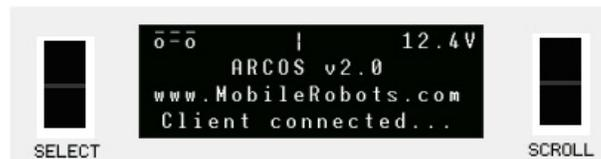
Figure 18. In normal mode, the LCD accessory displays operating status and client generated messages.
