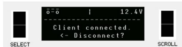
Figure 19. In interactive mode, the LCD lets you modify some operating features of the microcontroller.
