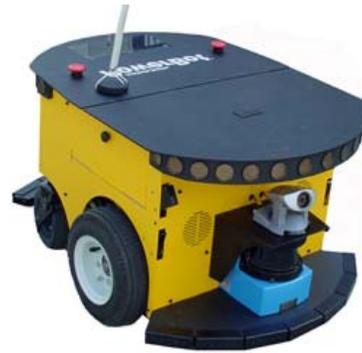
*Figure 8. PowerBot™ carries over 100 kg of payload.*
